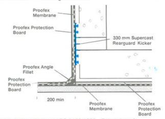
Note: Details based on BS 8102:1990 - Protection of structures from water from the ground
