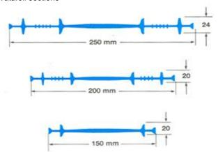
All centrally placed Supercast waterstops incorporate an eyeletted, reinforced edge flange. This enables them to be easily positioned by wiring to surrounding reinforcement.
