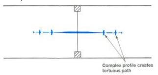
The Supercast range incorporates both of these principles. The products offer a fully continuous 4 bulbed design maintaining both the valve and tortuous path principles. These principles are maintained in the transition from Rearguard profiles in floors to centrally placed profiles in walls.
